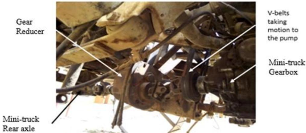
Plate 2: The Boom Sprayer underneath showing Gear Reducer installed in-between the vehicle gearbox and axle.
