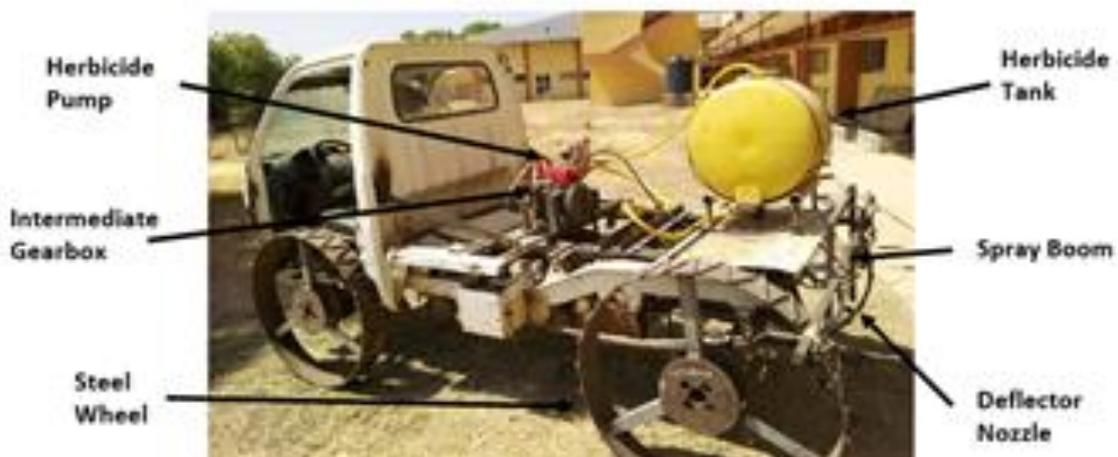
Plate 3. The Prototype Self-Propelled Cost-Effective Herbicide Boom Sprayer.
