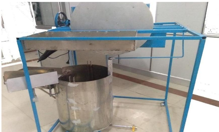
Fig. 2. Hand operated edible coating machine used for experimentation.
