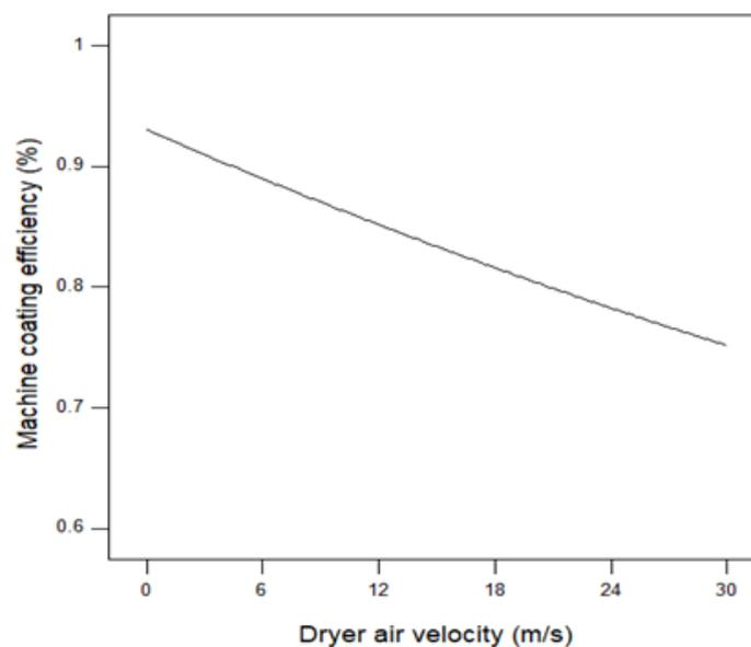
Fig. 3. Effect of dryer air velocity on machine coating efficiency.
